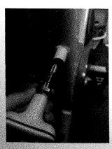
Insert the T handle Seat Post Locking bolt into the rear of the bike frame and tighten the steel bolt with a wrench: med-tight.
