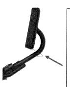
Mounting arm is hollow... insert cord through hole in base and pull through elbow. Leave about 12" of cord protruding from the elbow...
